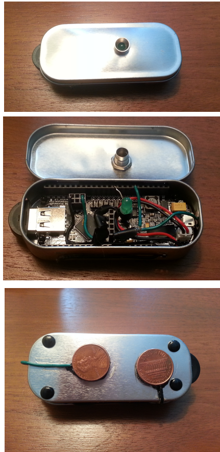
Figure 5: The IOIO board was mounted on a metal thin to enclose the battery and the Bluetooth dongle. The pennies functioned as galvanic skin sensors and were wired to the analog pin on the board. The circuit setup was similar to the one setup in the Arduino. Resistors and capacitor values were maintained. The LED indicates when the board is on use.
