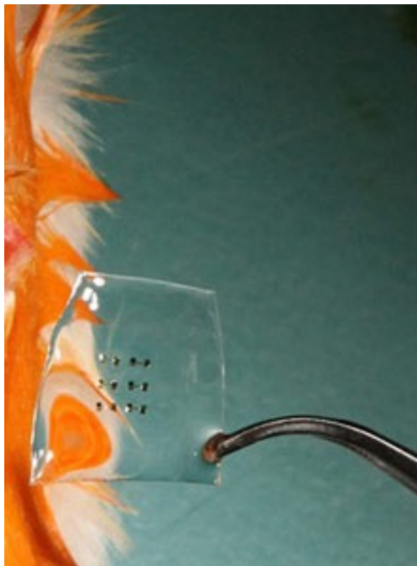
Figure 17: Clear silk film embedded with six silicon transistors as it is implanted in a laboratory mouse.
